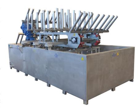
The equipment includes a filling and emptying system using manual valves. This equipment allows to control the scalding time of each animal, improving its quality. The temperature control is from high pressure to tenth of a degree centigrade.
